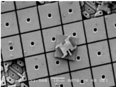
A scanning electron micrograph of a TI DLP chip.
