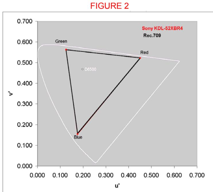
**Figure 2. 1976 CIE Uniform Chromaticity Diagram for the Sony unit.**
